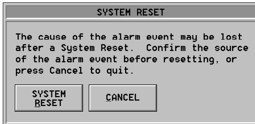
Figure 47 System Reset Window
